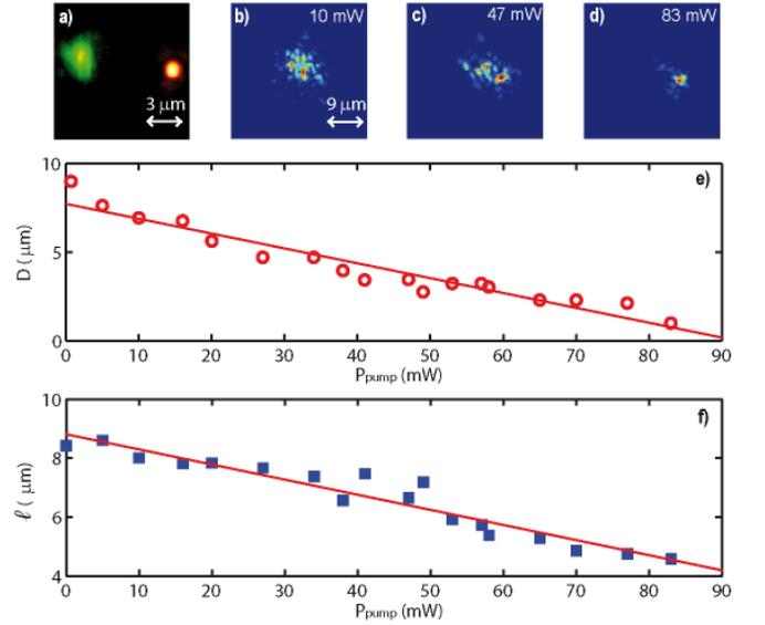
FIG. 4. (a) image of the entrance of the fiber (scale is  $3\mu m$ ); (b,c,d) fiber exit corresponding, respectively, to 10, 47 and 83 mW input power, the pump beam has been eliminated by a laser line filter (scale is  $9\mu m$ ); (e) displacement  $D$  versus  $P_{Pump}$ , fitted with equation 8 ( $D(0) = 7\mu m$ ;  $\frac{|\Delta n_2|z^2}{2n_0} = 0.01$ ); (f) localization length  $l$  as a function of  $P_{pump}$  and fit as in Fig. 2c.
